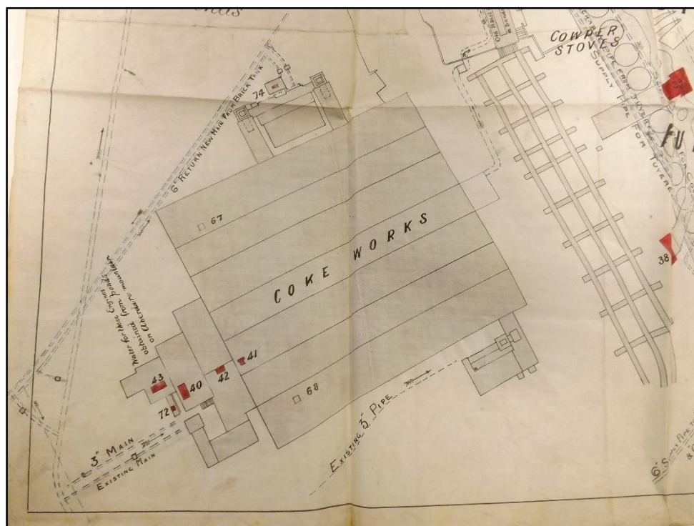
Plate 143. Plan of the Cyfarthfa Coppée coke oven dated 23rd February 1892. This is the form of complex prior to construction of the Sheppard washery in 1894/5. The red squares indicate the location of steam engines (Glamorgan Archives DG/F/9/10).
